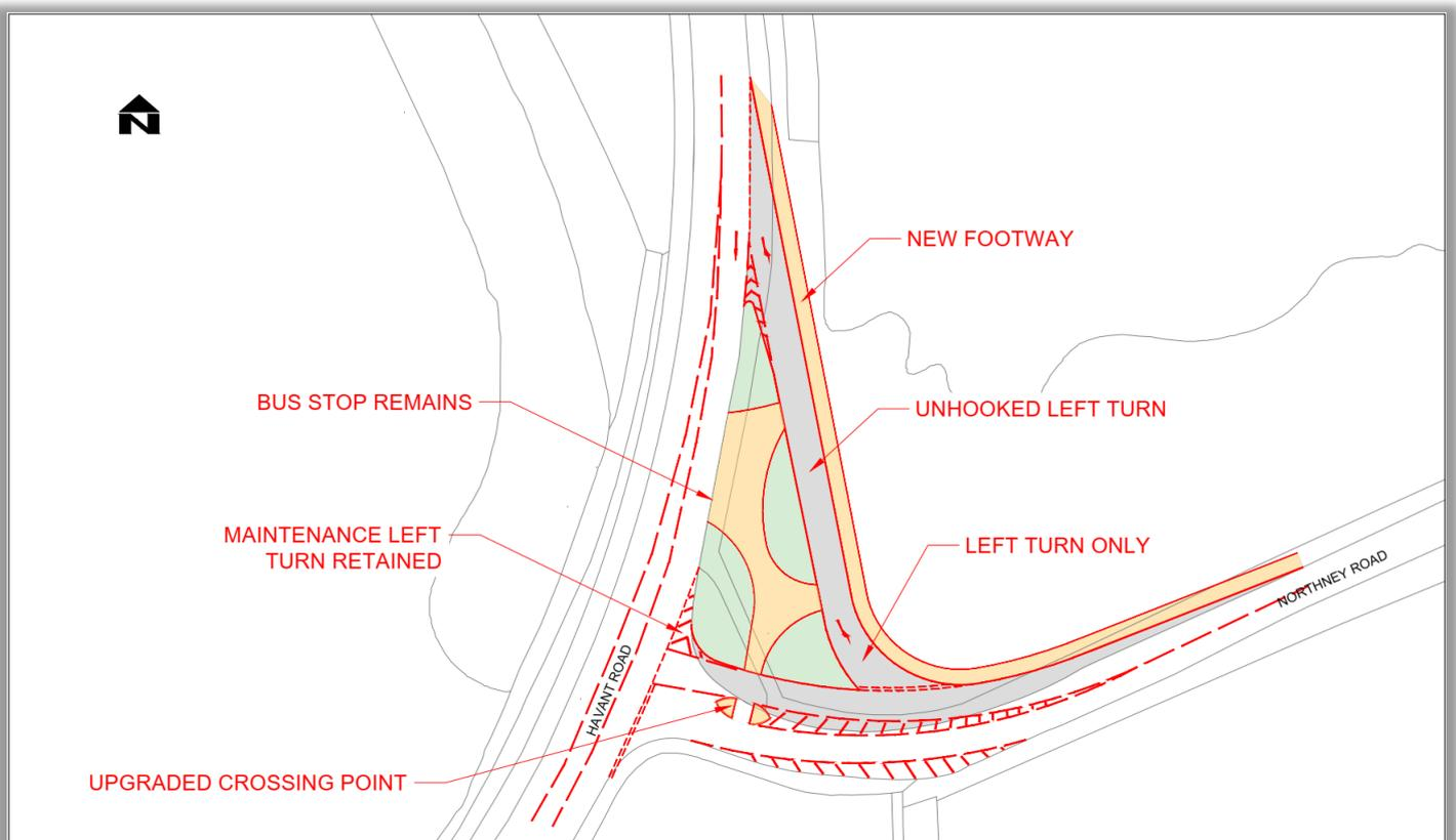
Figure 7: unhooked left turn at Northney Road
