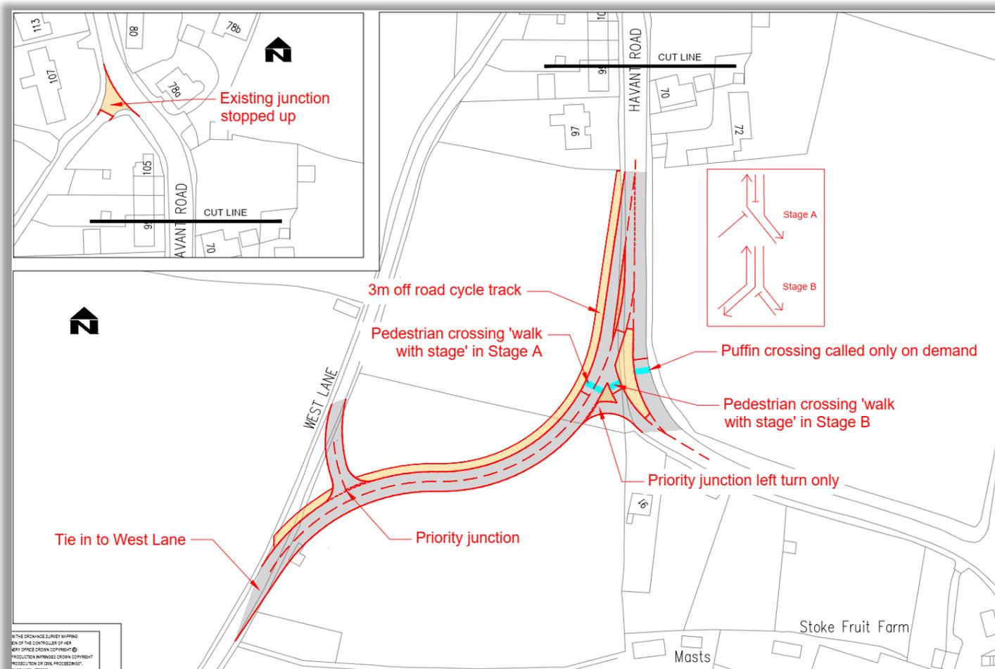
Figure 6: West Lane realigned and signalised junction – early provision would only require a priority junction
