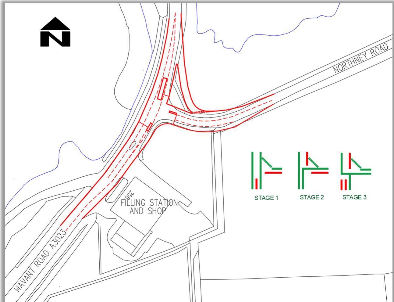
Figure 9: unhooked and signalised junction at Northney Road
