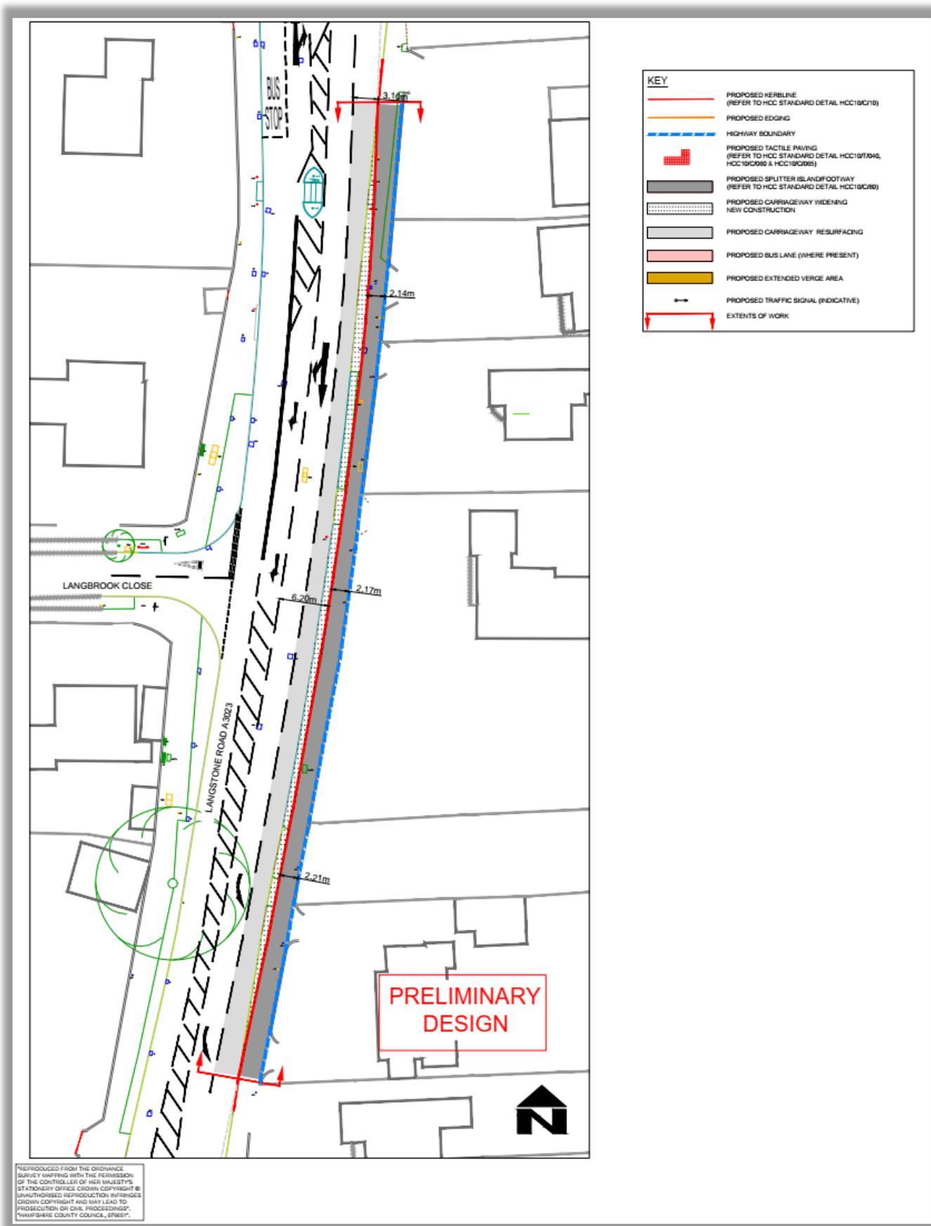
Figure 11: Extension of two-lane (southbound) in Langstone Road (phase 1 of possible improvements)
