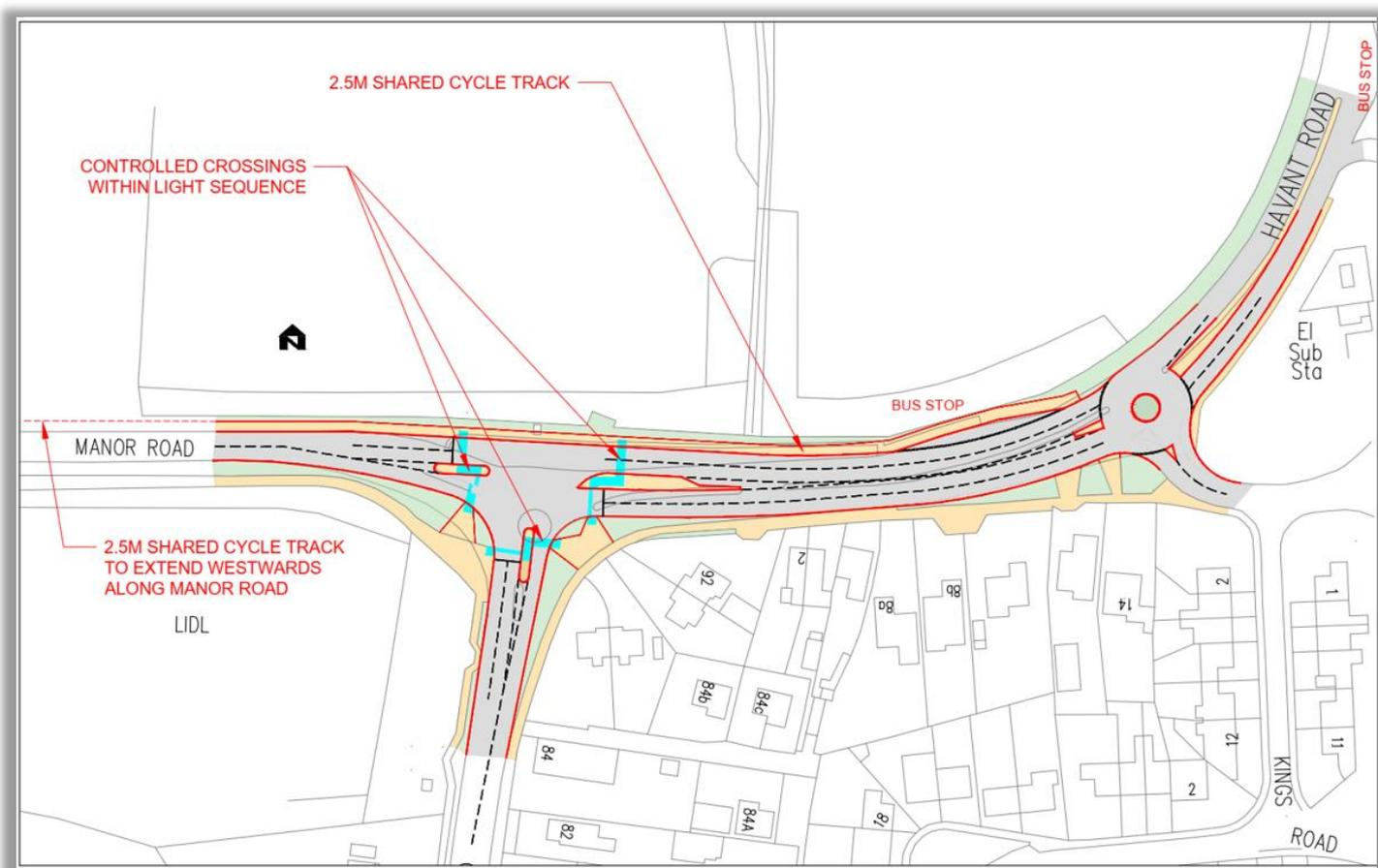
Figure 5: indicative layout for signalisation of Mill Rythe (Manor Road / Church Road / Havant Road) junction
