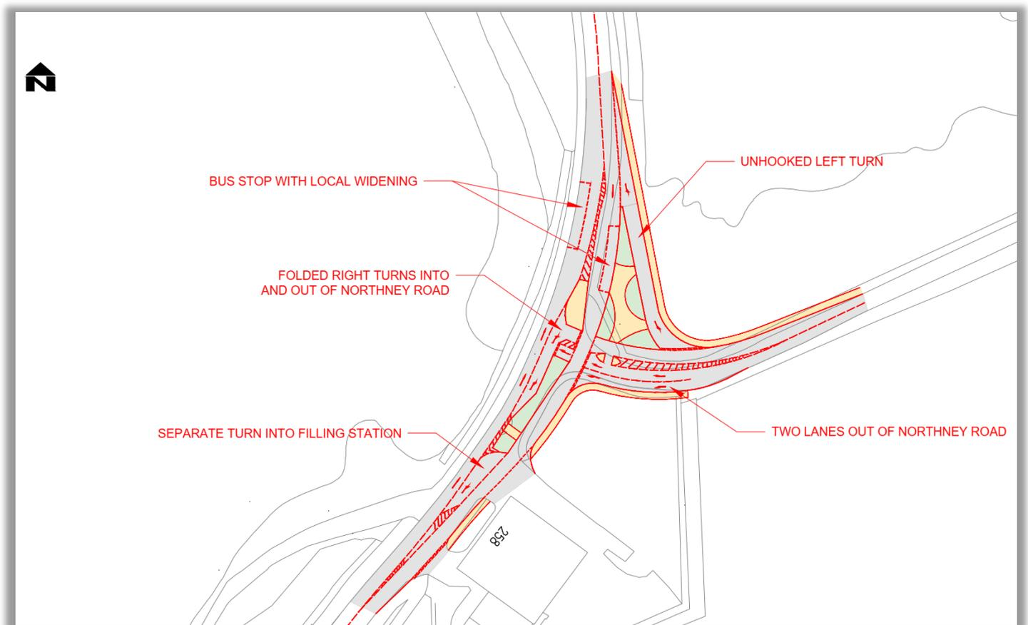
Figure 8: unhooked and folded turns at Northney Road
