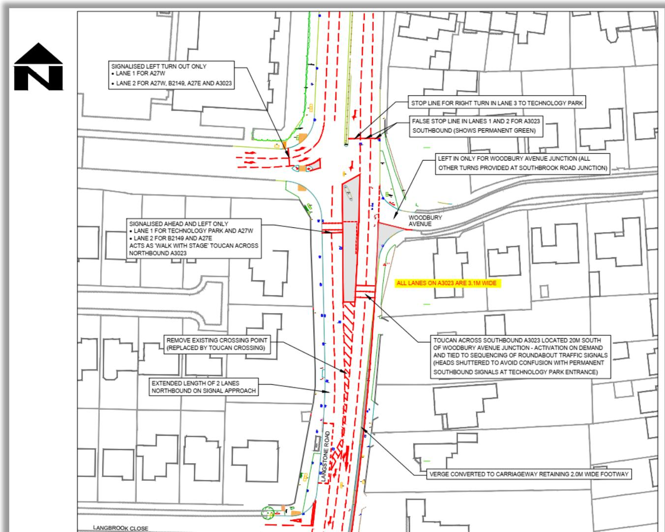
Figure 12: phase 2 Langstone Road with banned right turns, junction signalisation and pedestrian / cycle crossing facilities (only required late in Plan period and will be subject to further detailed testing and design)
